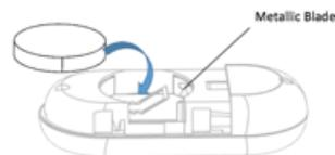
Press the metallic blade while installing the battery
